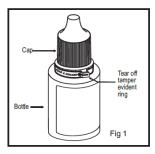
2. Before opening the dropper container for the first time, tear off the tamper evident ring to break the seal (Fig.2).
